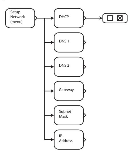
The **Setup Network Menu** allows you to configure various network parameters for the RMC-1.
