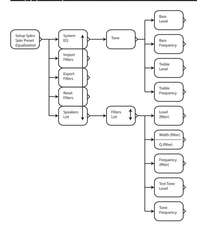
Once you have set the basic parameters for each preset (Speaker Size, Crossover Points, and Level Trims), you can use the RMC-1's powerful Parametric EQ filters and convenient Tone Controls to customize the sound just the way you want. Both the Tone Controls and the Parametric EQ filters may be used at the same time, giving you the precision and flexibility of Parametric EQ for detailed adjustments combined with the convenient sweeping tonal corrections offered by Tone Controls.
