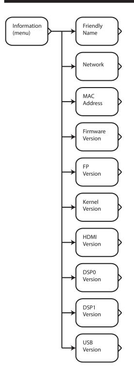
The *Information Menu* gives you access to information about the current Network configuration of the RMC-1, shows the versions of the currently installed firmware modules, and allows you to see the RMC-1's Friendly Name.
