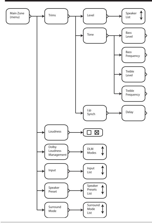
The *Main Zone Menu* contains the settings and controls typically used in the day-to-day operation of your RMC-1. These are settings that are typically chosen each time when viewing content; settings that remain in effect across multiple viewing sessions are accessed from the Setup Menu.
