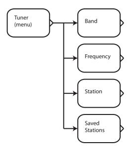
The **Tuner Menu** is used to select a station on the RMC-1's built-in high quality AM/FM tuner, and to create, rename, and delete station presets.
