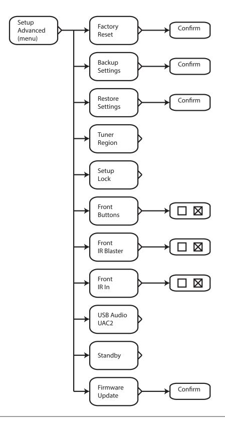
The **Setup Advanced Menu** allows you to configure various system operating preferences, including selecting a Standby Mode, and enabling various controls and remote control inputs and outputs. Firmware updates, and resetting your RMC-1 to factory defaults, are also initiated from this menu.
