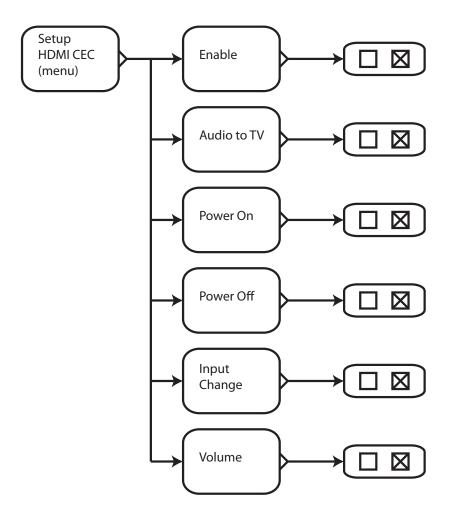
The **Setup HDMI CEC Menu** allows you to configure what types of CEC commands the RMC-1 sends and responds to.
