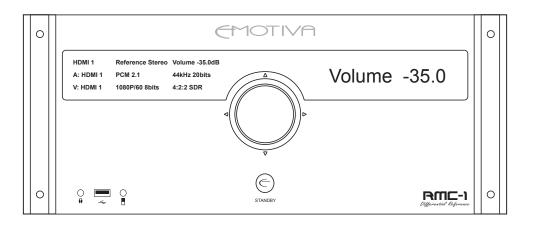
The front panel of the RMC-1 is dominated by a pair of large, bright, easy to read blue OLED displays. The displays can be set to any of six different brightness levels, including totally off. If the display is fully dimmed, it will illuminate for a few seconds when you press the Info button, and, when you activate the Menu, the display will illuminate for as long as you are using the Menu.
