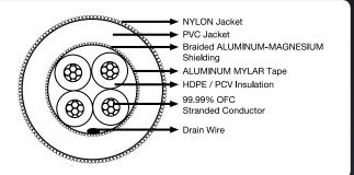
TUD-20 Type A-to-B USB 2.0 Digital Cable [available terminated] Because music signals are continuous streams of data, in case of any disruption or errors during transmission through a USB cable there is no chance to replace any missing part of the audio signal. It is crucial to use a high grade USB cable that preserves more information and significantly improves sound quality.
