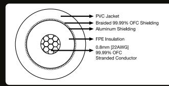
Ultra-high purity 0.8mm [22AWG] 99.99% Oxygen Free Copper conductors, Precision machined, low-profile RCA connectors with gold-plated contacts
