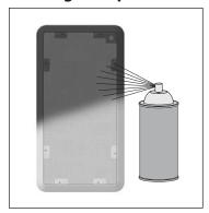
The white plastic frame and the metal grille may be left as is, or painted to match your décor. You can paint the frame before or after it is installed in the wall. Spray painting (using slightly thinned paint) is the best method to use for painting the grille. After painting the grille, use air pressure to "blow out" any grille holes that are filled in with paint.
