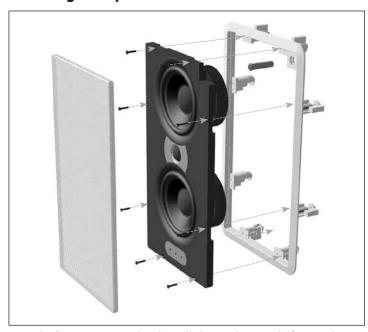
Once the frame is mounted in the wall, the speaker simply fits into the frame. Note that there is a gasket around the edge of the MDF baffle. This gasket ensures an airtight fit between the baffle and the frame. Therefore, the baffle may fit tightly in the frame. This is normal.
