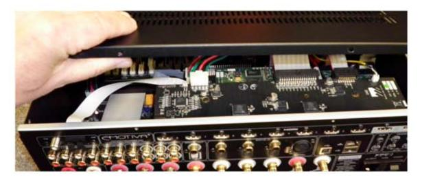
NOTE: Several different sizes and types of screws are used in the XMC-1. When you remove the screws, be sure to keep track of which screws are removed from each location so you can replace the correct screws in their proper locations later.
