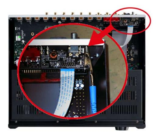
NOTE: The connectors inside your XMC-1 may be secured in place with a small dab of flexible adhesive to prevent their loosening during shipping. If you have trouble removing connectors, try gently wiggling them from side to side to loosen then. If necessary, use a small screwdriver or knife to carefully scrape away some of the adhesive. When unplugging a connector, always apply pressure to the connector itself if possible, and use extreme care if you pull on the cable to remove it.
