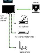
No additional network cable required betw net access and AV com
