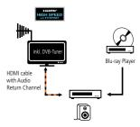
No additional audio cable required betwee IV and AV reveiver.
